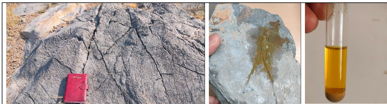
Figure 11. Grey dolomitic limestone with elephant skin weathering near Barsingha village (A). B & C show the Sapiro test result, indicating phosphate content.
